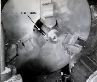
Shim under one jaw holds piece off center. After turning, the eccentric end is drilled and tapped for the \frac{1}{4} "-20 retaining screw.
